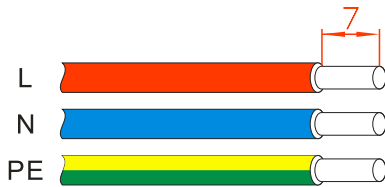
Figure3-20 Stripping diagram of AC output (unit: mm)
