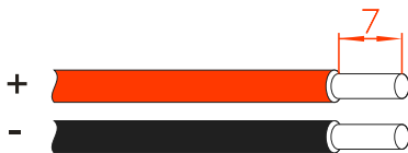
Figure3-15 Stripping diagram of DC input (unit: mm)
