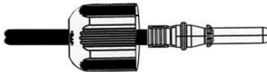
Figure4-13 Crimp the negative metal terminal
