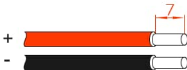
Figure3-15 Stripping diagram of DC input (unit: mm)
