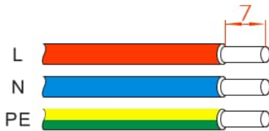
Figure3-20 Stripping diagram of AC output (unit: mm)
